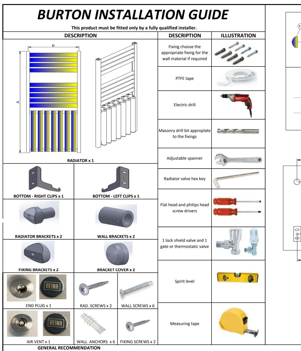
Before fitting the radiator it is necessary to wash out the heating system to remove any existing mud, scale, work residues, traces of flux, oil, etc.
