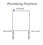
Vertical mount All Dimensions are in mm Max.Working Pressure: 10 Bar Max.Working Temperature: 95° C Inlet / Outlet: 1/2" BSP Fuel: E/H/D
