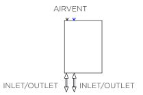
Vertical Mount All Dimension are in mm Max.Working Pressure = 10 Bar Max.Working Temprature=95° C Inlet / Outlet : 1/2" BSP Fuel: H
