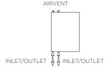
Vertical Mount All Dimension are in mm Max.Working Pressure = 10 Bar Max.Working Temprature=95° C Inlet / Outlet : 1/2" BSP
