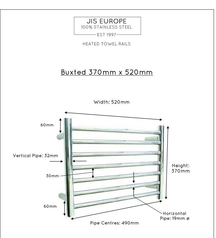
Overall Projection: 117mm\* Pipe Centres from the Wall: 102mm\* \*When using short brackets, projection and pipe centres from wall will be reduced by 25mm.
