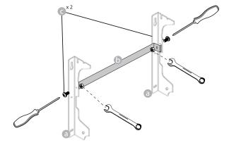
2. Choose the radiator position, refer to the warnings of paragraphs 1, 2 and 2.1. Depending on the position chosen, place the bracket a on the floor
