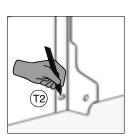
6. Depending on the type of wall, select suitable screws and dowels, the screws and dowels supplied may not be suitable for the type of wall of your home. Drill as indicated by the holes marked and then insert the blocks in the wall.
