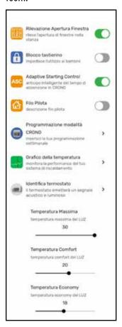
Programming from APP follows the same criteria as described for the radiator, with the possibility of setting three comfort operating time slots for each day; instead, it is not possible to copy programs from one day to another as in programming from radiator.
