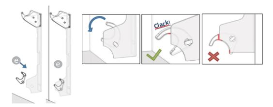
Position the radiator by leaning it on the upper part of the brackets and then rotating it. Push the radiator until it is automatically locked by lower plastic clamps (e).
