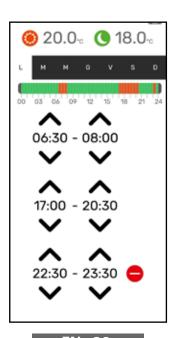
The APP also allows displaying the trend of the daily, the previous day or the previous week ambient temperature, and comparing it with the desired settings, so as to adapt the most suitable settings to your needs and manage consumption.
