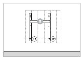
5. Using a spirit level, check that the bracket is straight and mark the position of the two upper holes (1) and (12).
