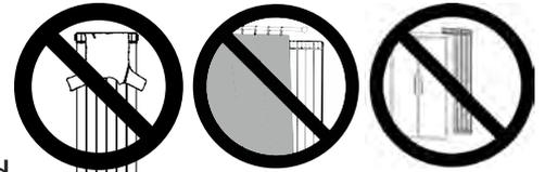
The radiator must be secured to the wall using the supplied mounts..
