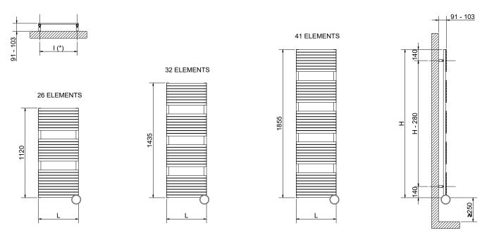
(\*) Pipe center (I) measure of the fixing kit  $\hfill O$  The general footprint has to be calculated considering the thermostat height
