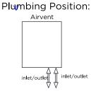
All Dimension are in mm Max.Working Pressure = 10 Bar Max.Working Temprature=95° C Inlet / Outlet : 1/2" BSP
