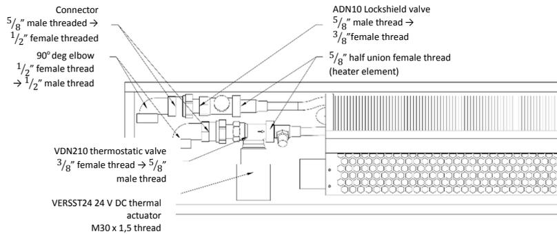
For VKN1 heater thermostatic and lockshield valves should be DN 10 diameter. E.g. Siemens VDN210 as a thermostatic valve and Siemens ADN10 as a lockshield valve. Connector 5/8" male threaded -> 1/2" female threaded is as standard heater equipment.
