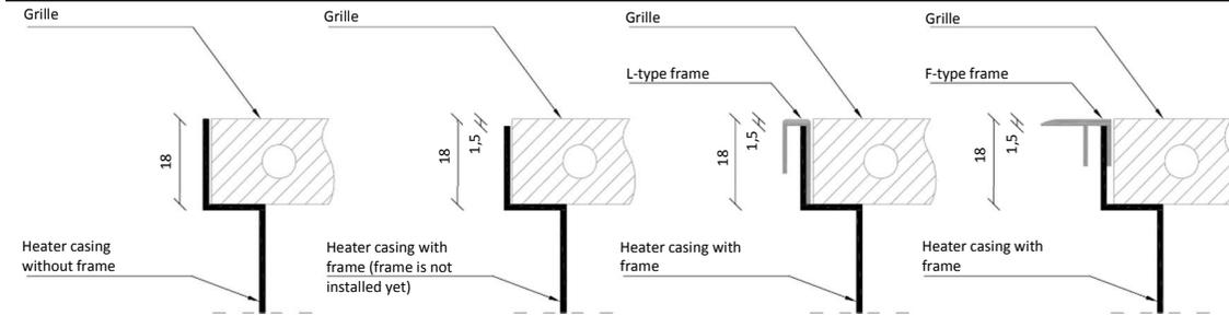
The height of the casing edge depends of the frame type. It is recommended to order heater with frame at the same type (if heater is going to be finished with frame).
