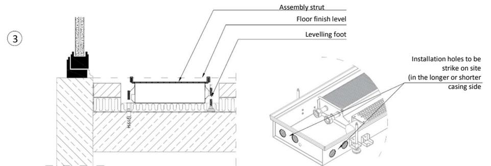
**10. Install the heater casing in the trench**
