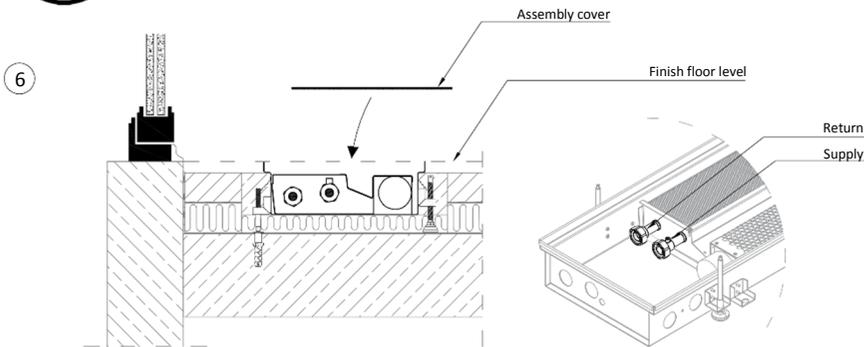
**13. Do the hydronic and electric connections to the heating kit**
