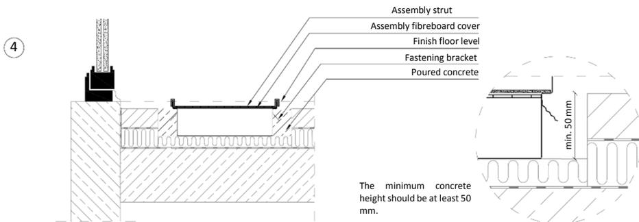
**11. Do the hydronic and electric connections, pour the concrete around the casing**
