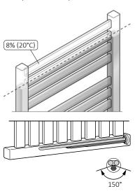
When installing the heating element horizontally, the single tube (capillary) where the temperature sensor is located, should be positioned to be as close to the bottom of the radiator as possible.
