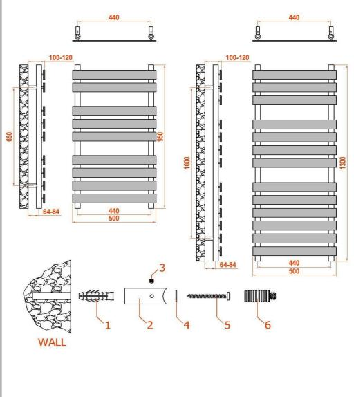
The radiator should closer than 50mm below any overhanging surface (i.ei shelf) and no lower than 100mm from the floor. Transfer the bracket drill position Drill the wall and insert wall anchors (1) or other suitable fixings). Put the brackets (2) on the wall and screv them to the wall anchors (1) with fixing screws (5) and washers (4). Screw the brackets (6) onto the nuts welded on the back of the
