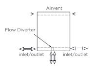
When mounting vertically, please observe that the collector fitted with a flow diverter is mounted at the bottom. This can be verified by visually checking or by referring to the installation diagram
