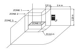
The national rules on installing electrical equipment in the bathroom must be scrupulously respected. The electric radiators must be always installed outside zone 1 and 2.
