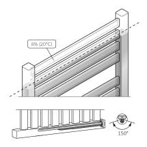
When the heating element is installed horizontally, it must be rotated to such an extent that the single tube, which houses the temperature sensor, is positioned as low as possible.
