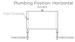
When mounting horizontally, please knock through the centre hole of the diverter using a suitable rod. Please remove the disk if it comes loose and can be removed from a tapping.
