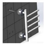
Unthread the cap to see the visible mounting seat, level the installation mounting size and mark installation holes by pencil
