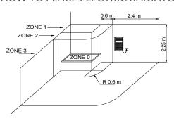
The national rules on installing electrical equipment in the bathroom must be scrupulously respected. The electric radiators must be always installed outside zone 1 and 2.
