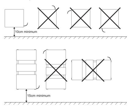
**NOTE:** Electric towel radiators are designed to be covered safely. However, to ensure that your appliance works efficiently, you are advised not to cover it completely. Doing so will increase the temperature and cause the internal cutout to turn off the appliance.
